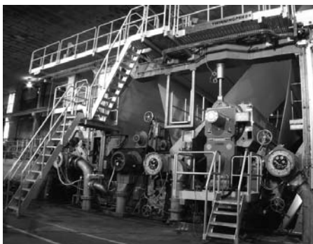
Linear pressures up to 1,200 kN/m thanks to the TwinningPress™ shoe press
