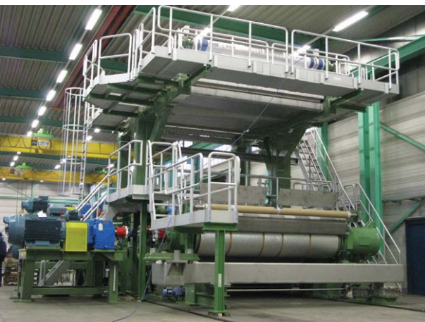
A usual Bellmer procedure: complete workshop assembly of the press section
