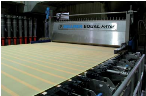
The heart of the paper machine: the headbox
