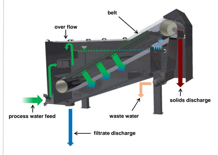
The design of the belt grants a **high separation efficiency** and **COD reduction**. The transport of the belt is carried out by a special vulcanized toothed belt.
