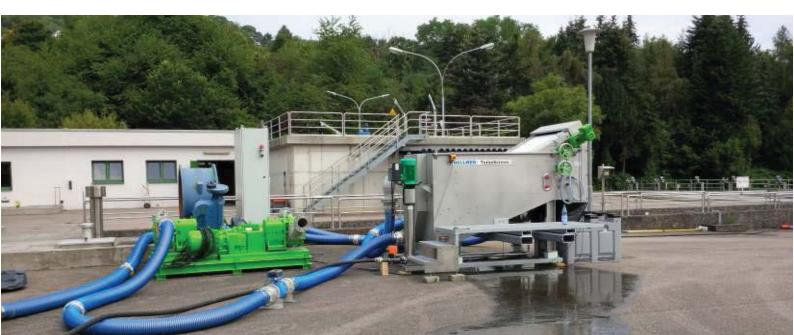
Adwantages ✓ reduction of suspended solids high COD reduction high throughputs Iow energy costs compact design clean and enclosed operation easy cleaning and handling TurboScreen Separation Technology
